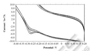
Figure 3: CV showing peaks for different concentrations of MB-DNA complex in 200 mM KCl, Scan rate: 0.1 V/s.
